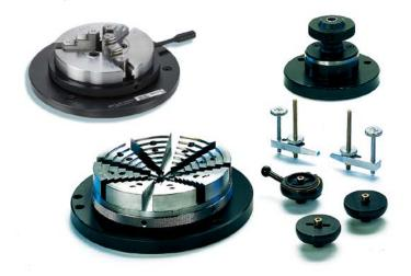
Three-jaw chuck, dia. 100 mm with mounting flange of dia. 160 mm, reversible jaws for external and internal clamping. Clamping range: external 1 to 100 mm, internal 36 to 90 mm. Total height with flange 47 mm. Adjustment by means of rotating ring.
