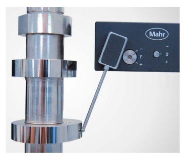
freely selectable form factor between contour representation and the representation of the toler-ance band deviation. More cam-specific characteristics such as stroke curves and cam angle can also be evaluated. Special assessments such as the acceleration curve and the velocity curve calculated from the profiles are also included with the scope of this **Quick&Easy CAM.**
