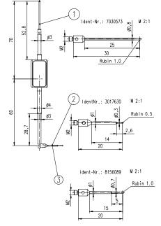
for measuring small workpieces, consisting of a probe arm
