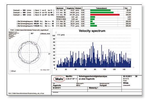
Manufactured parts for roller bearings come out of machining processes with roundness and waviness deviations from their ideal geometry. In components for high speed bearings (such as those found in computer hard disks, for example), form deviations of raceways from the ideal, smooth circle can lead to uneven running, development of noise, and reduced service life due to increased wear.
